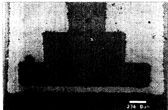
Fig. 5. Optical micrograph for the MR element part of the patterned discontinuous multilayer with the structure of Si/Ta(40Å)/Ag(20Å)/NiFe(15Å)/[Ag(45Å)/NiFe(15Å)] n /Ag(20Å)/Ta(100Å).
