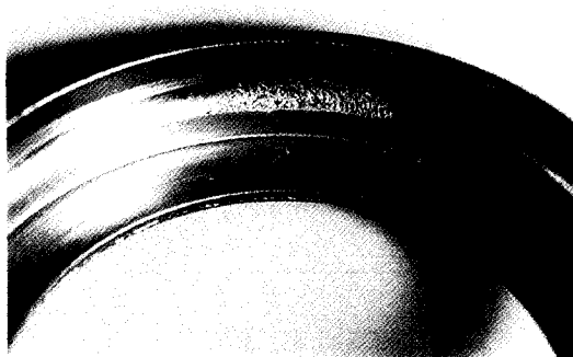
Fig. 15. Fatigue flaking on outer raceway.
