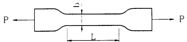
Fig. 1 Geometry of the tensile test specimen of the rotary screen
