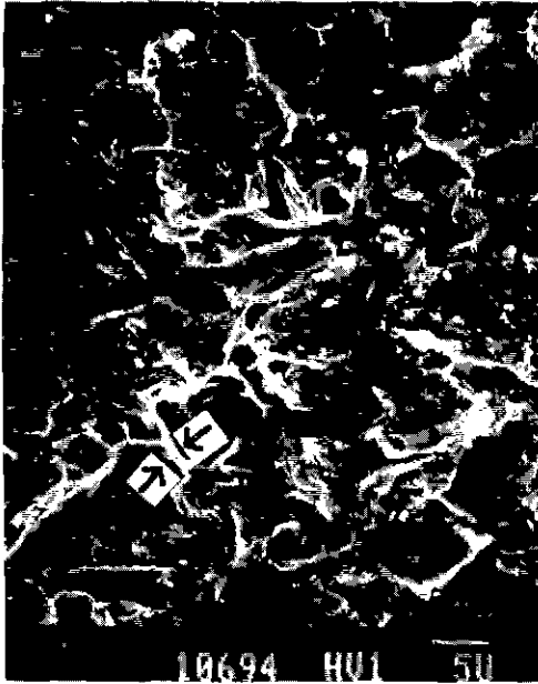
Fig. 8. Fracture surface of SiC-Al alloy composite infiltrated at 1400°C-4 hrs
