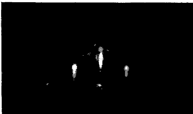
Fig. 3. RHEED pattern of the film deposited on a Si(001) substrate at 930°C.
