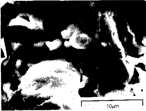
Fig. 1. Scanning electron micrograph of MoSi 2 powder used in present study.
