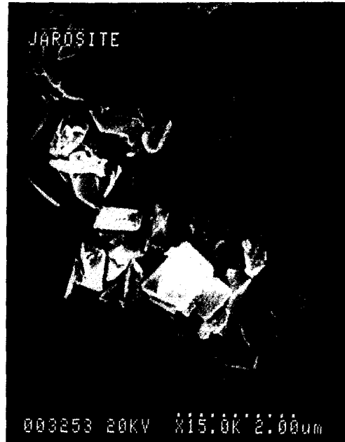
Fig. 4. Scanning electron micrograph of jarosite from Gimhae series (B2 horizon).
