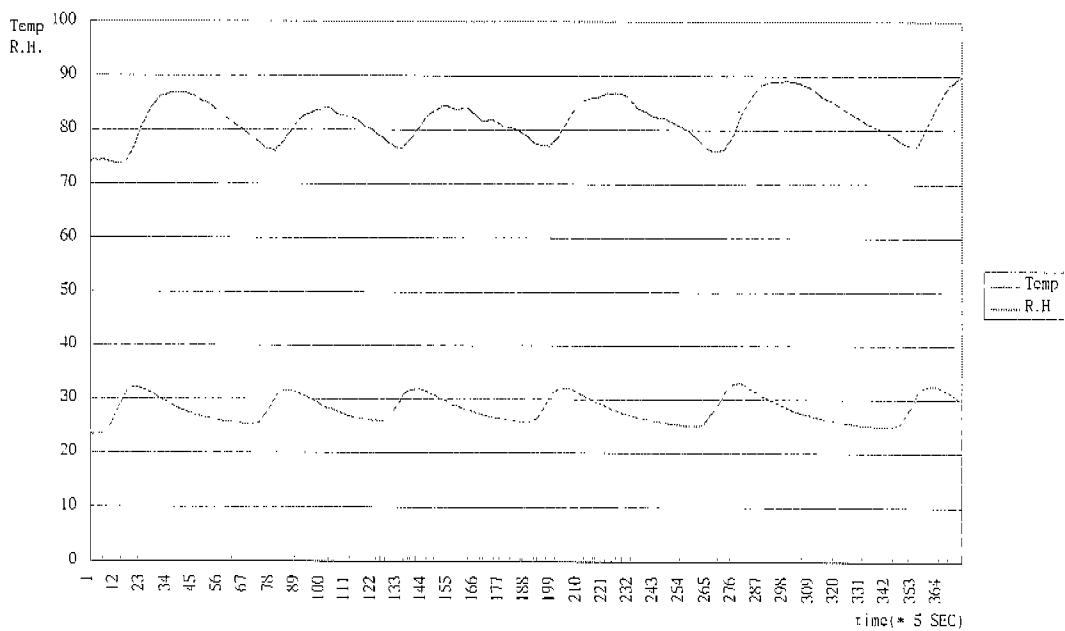
(b) Conventional system that control temperature and humidity separately (Reference Temp. : 30°C, Reference R.H. : 84% J(T) : 993.7 J(H) : 1520.0)
