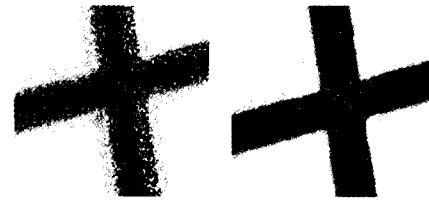
FIG. 6. Anomalies associated with flat objects. The composed image( left) is noisier than the best focus image. The object was a "+" on a tilted plane.
