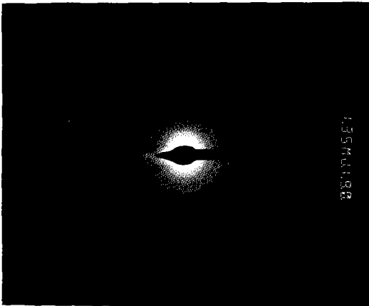
Fig. 5. SADP Micrographs of TiO 2 Coated on Graphite. (a) Graphite, (b) TiO 2 .
