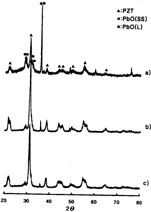
Fig. 7. XRD patterns of PZT powders prepared at 2 m KOH solution as a function of temperature. a) 140°C, b) 150°C, c) 160°C.
