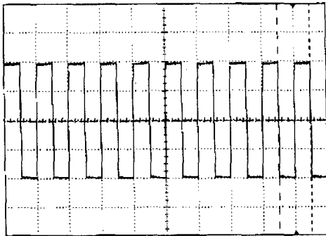
Horizontal : 10usec/div Vertical : 6V /div (b)
