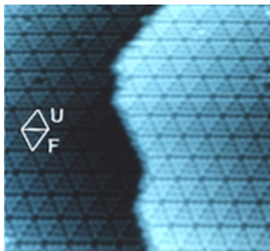
Fig. 1. 7\times 7 structure of clean Si(111) surface. Scan area 270 \text{ \AA} \times 280 \text{ \AA} , V_S = -2.5 \text{ V} , I_t = 0.5 \text{ nA} .
