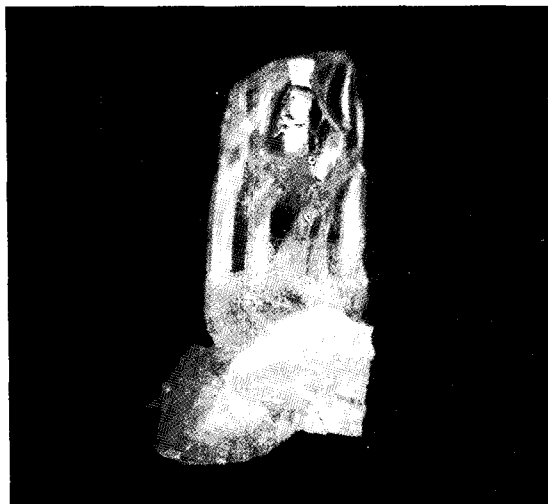
Fig. 1. A separated column of yttria stabilized cubic zirconia.
