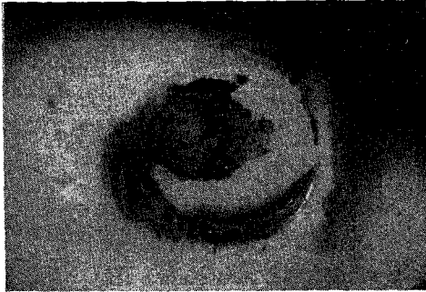
Fig 3. SMPDA :Mixed failure
