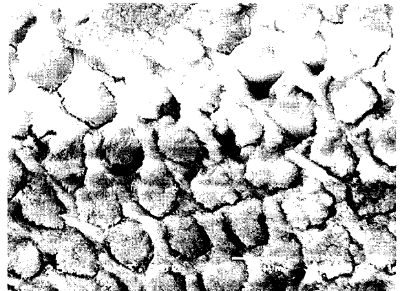
Fig. 5. Scanning electron micrograph of enamel surface after etching with 38% phosphoric acid for 60 seconds. Areas showing preferential loss of prism cores where prism peripheries are prominent. (original magnification \times 3,500 )
