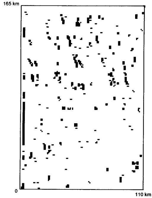
Fig. 5. Indicator map of slope in the study area. (white : maximum slope < 10%, black : maximum slope ≥ 10%, 1 km×1 km grid)
