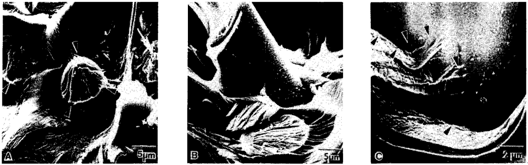
그림 14. SEI of a glass fiber reinforced nylon showing (a) nearly lateral failure across the matrix and fiber due to excellent adhesion between the fiber surfaces and the matrix, (b) classical brittle fracture (arrow), and (c) adhesion of the matrix at the fiber surfaces.
