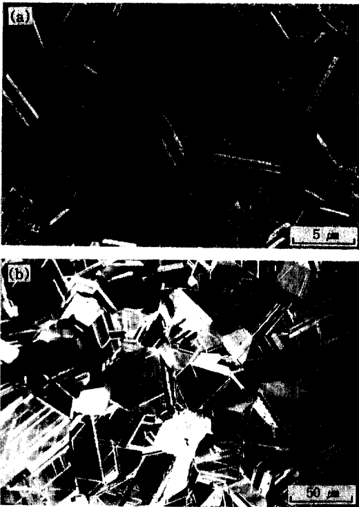
Photo 1 Variation of \epsilon martensite morphology with solution treatment temperature in Fe-17%Mn alloy. Annealed at (a)700℃ and (b)1000℃ for 30min. after 60% cold rolling.
