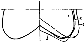
Fig. 2 Comparison of Bowl Geometry for Different Aspect Ratio(d c /H)
