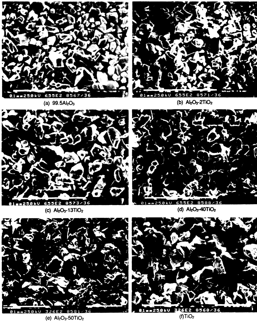
Fig. 2 SEM micrographs showing the morphology of the ceramic powders for plasma spraying
