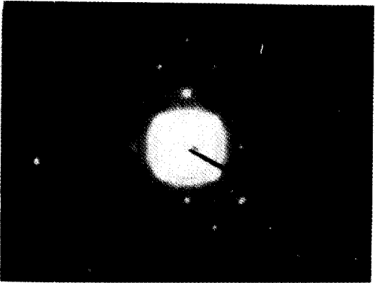
Fig. 4. Transmission electron diffraction pattern for 5 nm cobalt thin film deposited on silicon.
