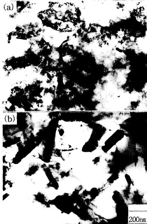
Fig. 5. TEM micrographs of mechanically alloyed Al-8wt.%(1Ti+1Zr) after isothermal aging for 100hrs; (a) 400°C (b) 510°C.
