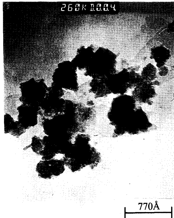
Fig. 3. TEM micrograph for YIG particles prepared with the initial concentration of 0.096M.
