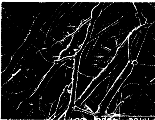
Photo. 1. Microstructure of magnetic fibrous polymeric filter (×100), — 100 μm.
