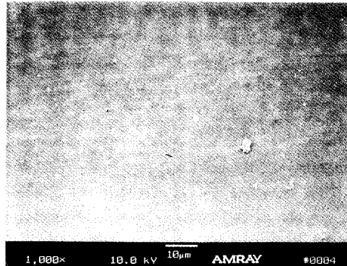
Fig. 6. A SEM micrograph showing a run-in film surface on the right hand; and an initial rough film surface on the left hand.
