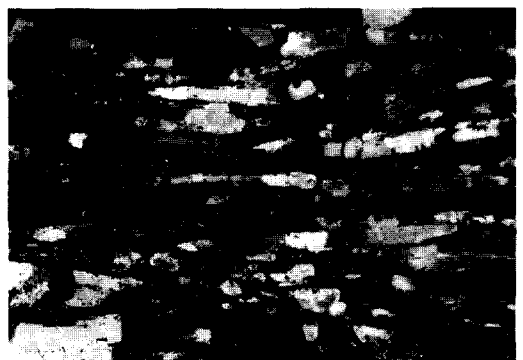
Fig. 5. Mylonite in the Jaesan formation formed by Jaesan Thrust. Crossed nicols, x40.
