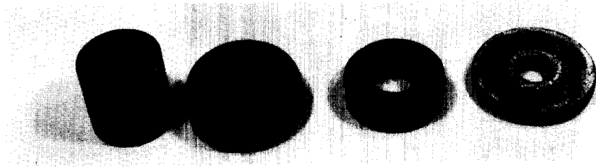
Fig. 6 Specimens for compression and ring compression tests
