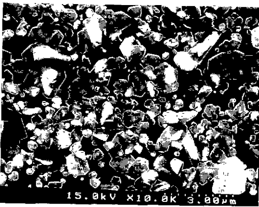
Fig. 11. SEM microstructure of reaction bonded silicon carbide by slip casting method.
