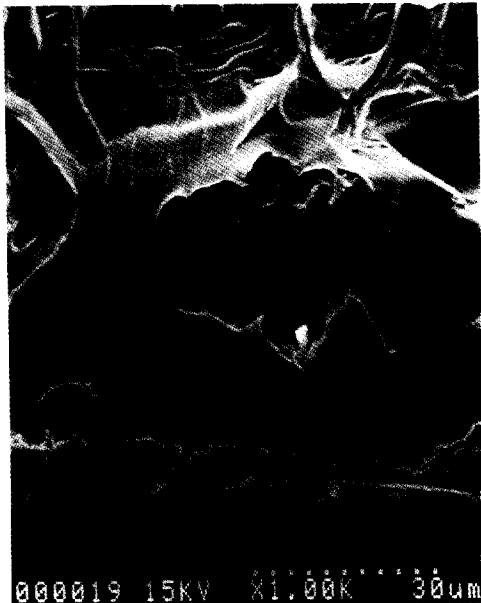
Fig. 2. Electron micrographs of the cross-section of SB1 membrane. Magnification: 1,000X.
