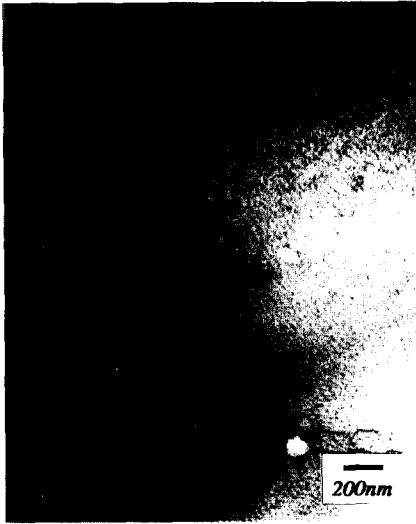
Fig. 8. TEM of the Fe-rich particle in a TiB 2 grain. The micrograph also shows the formation of dislocations.
