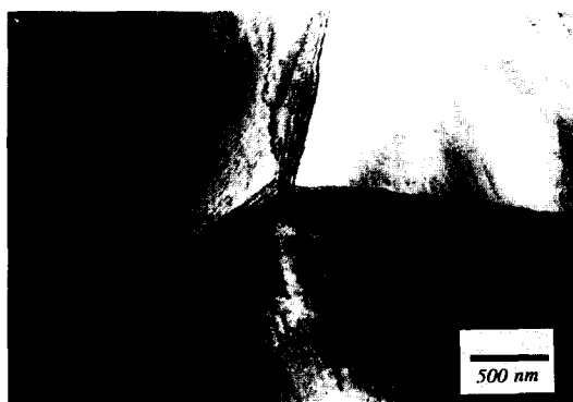
Fig. 1. TEM of the typical grain edge in TiB 2 .
