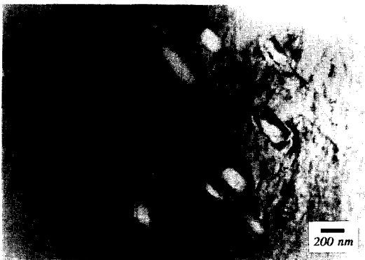
Fig. 5. TEM of the Fe-rich particles distribution in a TiB 2 grain.
