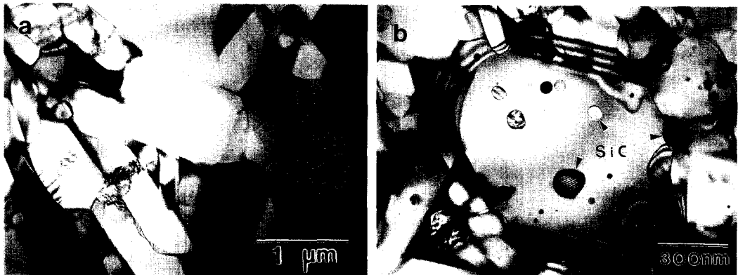
Fig. 3. TEM micrographs of monolithic Si 3 N 4 , (a) and Si 3 N 4 /30 vol% SiC nanocomposites (b).
