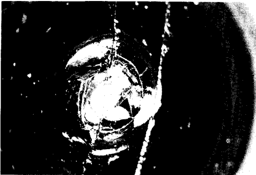
Fig. 3. Growth striation on the surface of \text{LiNbO}_3 crystals.
