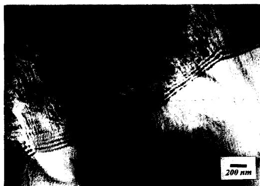
Fig. 4. TEM of a high angle grain boundary in TiB 2 .
