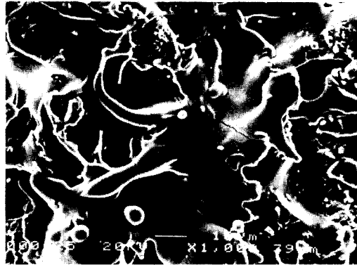
Photo. 4 Morphology of cracks on the top coat
