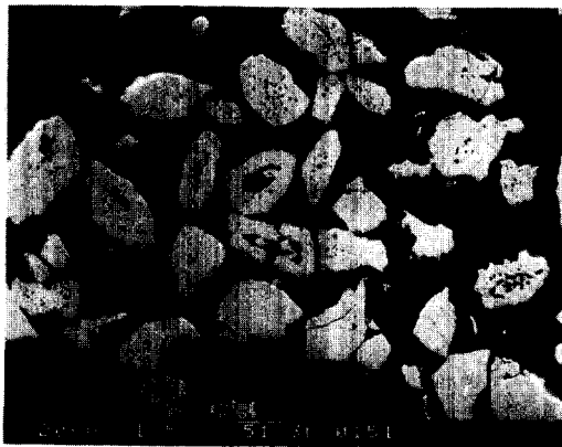
Photo. 2 The cross-section of Cr_3C_2 -NiCr powder
