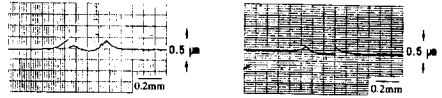
(b-1) Static indentation (b-2) Impact (V=44.4 m/s, P=735 N, D 2 =0.328 mm) D 2 =0.270 mm
