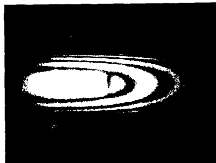
Fig. 7 Fringe pattern of circumferential-defective tube
