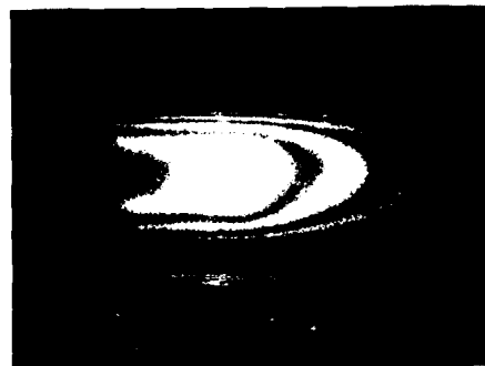
Fig. 6 Fringe pattern of axial-defective tube
