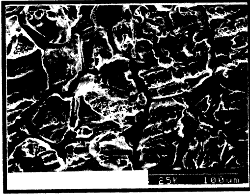
Fig.10 SEM photography of intergranular corrosion tested sample No. 2
