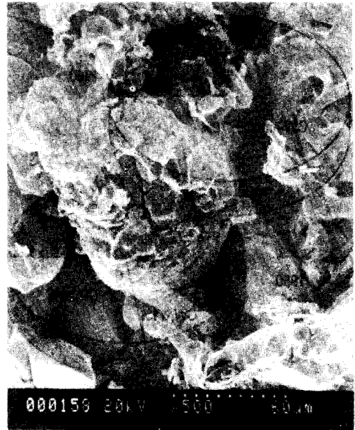
Photo. 1 Cross section microstructure of flame thermal sprayed Al_2O_3 coatings.
