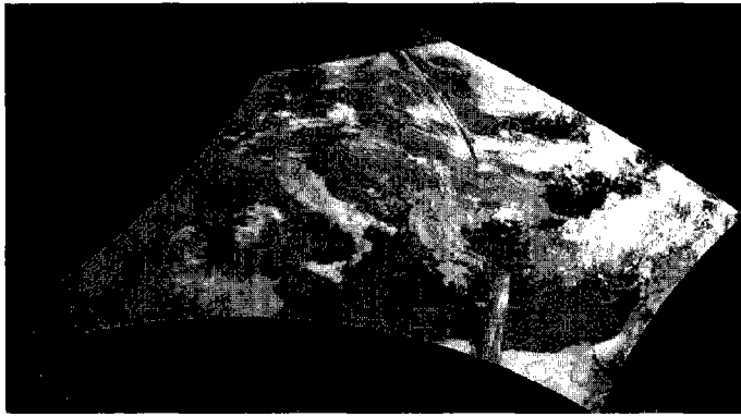
Fig. 6. Image projected to latitude and longitude grid after radiometric and geometric correction
