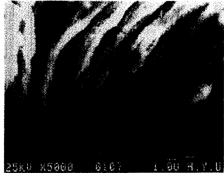
(da / dN=2.28 \mu\text{m} / cycle, \Delta K=129.88\text{MPa} \cdot \text{m}^{1/2} )
