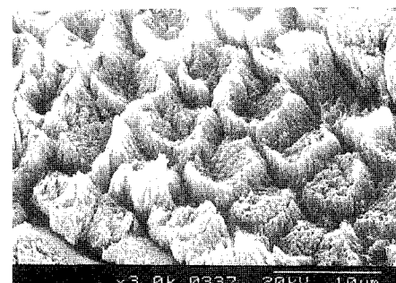
H: saliva contamination, 10sec. re-etching.*
