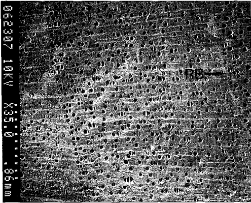
Fig. 5. Cross Section of Acer spp(SEM)
