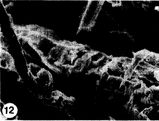
Fig. 12. Morphological features of fiber and adhesives after internal bond test. Fibers were encrusted with adhesives ( \times 400 ).
