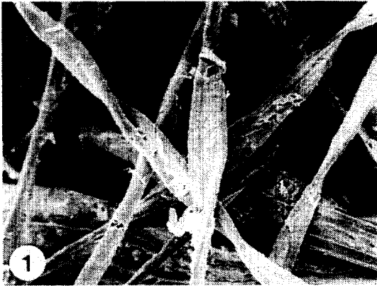
Fig. 1. Softwood MDF fiber at low magnification. Fiber twisting and surface loosening was occurred ( \times 200 ).
