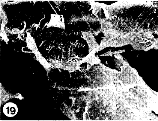
Fig. 19. Fiber contact area where the adhesion occurred. Arrow(→) shows adhesion site ( \times 2,000 ).
