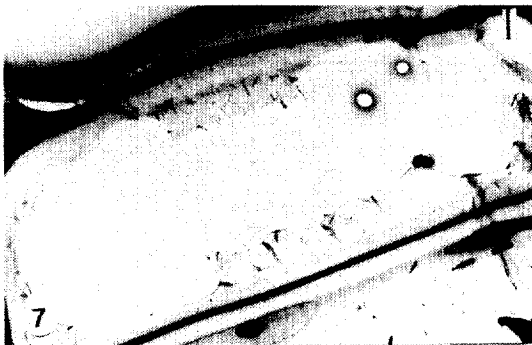
Fig. 7. The thinning and dentate erosion of the secondary wall are progressed from lumen toward compound middle lamella (bar: 2 \mu m).
