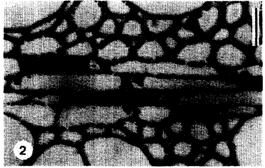
Fig. 2. The most typical changes are cracks of the secondary wall from compound middle lamella (bar: 10 \mu\text{m} ).
