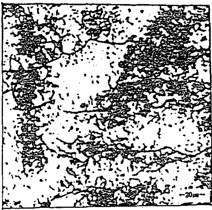
austenitic 304 stainless steel (Na 2 CO 3 : 0wt%)
