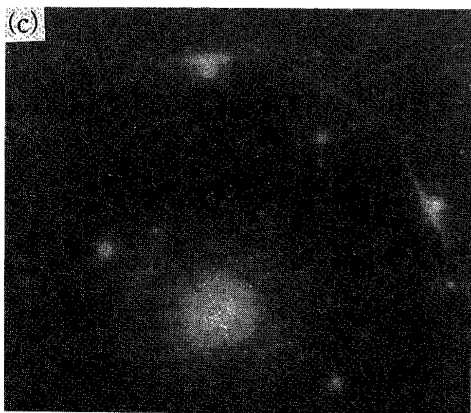
Photo 4. Transmission electron micrographs of single roll melt spun Al-6.0at.%Be alloy. a) bright field image, b) dark field image, c) SADP, d) solution of(c)
