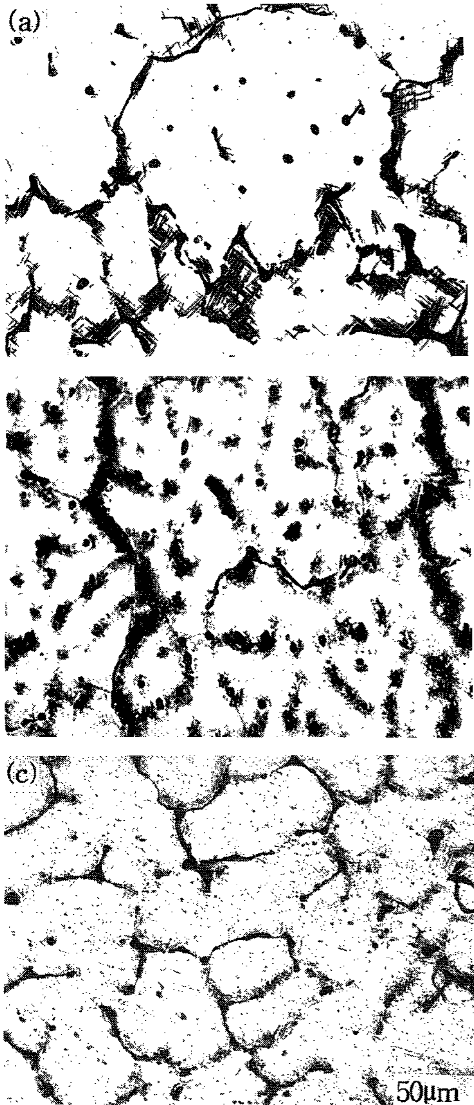
Photo 1. Optical micrographs of Al-Cu-Li-X (In, Be) alloys as cast condition (a) 2090 (b) 2090-In (c) 2090-In, Be
