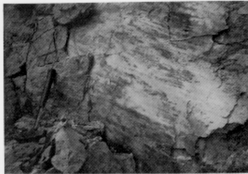
Fig. 6. Dextral strike-slip fault which is NNE direction at the basement of Tertiary basin.
