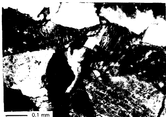
Fig. 11. Laumontite (L) pore-fill cement and replacement of plagioclase grain (Pl). Note optical continuity of laumontite cement to replacement across the original plagioclase grain boundary delineated by the C/S clay. Sample 5-61, 2335.7 m. Crossed nicols.
